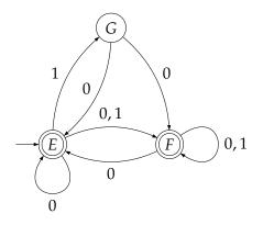
3. Let  $\Sigma = \{a, b, c\}$ . Using the systematic method described in class and textbook convert the following nondeterministic state transition diagram into a deterministic transition diagram:
