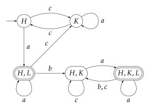
The only accepting state in the original automaton is *L* and so the accepting states in the deterministic automaton are the two that contain *L* namely,  $\{H, L\}$  and  $\{H, K, L\}$ .
