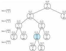
Substantially smaller tree than in the case of breadth-first branch & bound.
